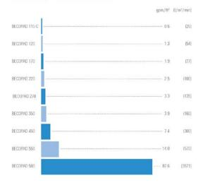
Conditions:  $\Delta p = 14.5 \text{ psi}$  (100 kPa, 1 bar), Medium: Water at 68 °F (20 °C)
